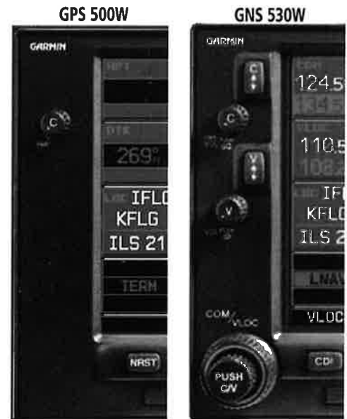
On the GNS 530W, the large and small left knobs allow you to tune the desired COM or VLOC frequency.
