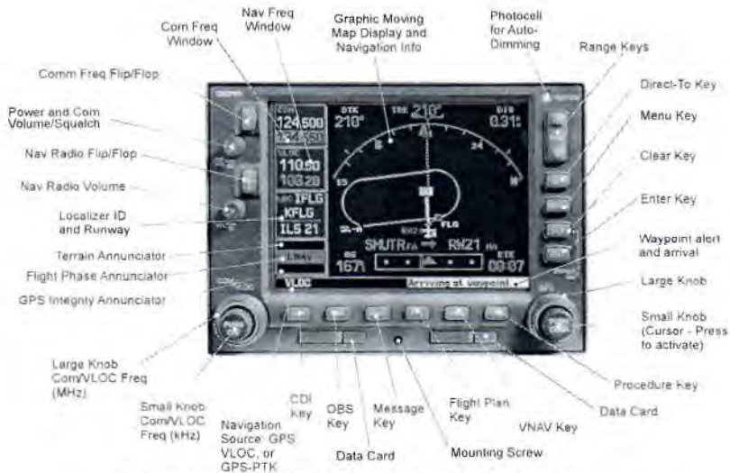
Figure 1 - 530W Series Control and Display Layout
